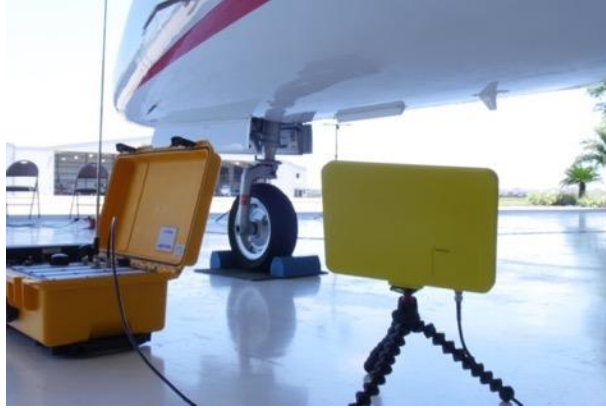
ARTS 7000 Pulse antenna showing good alignment with an aircraft bottom antenna.
