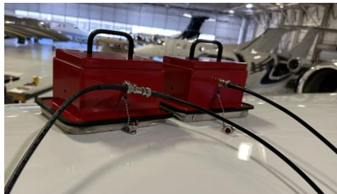
ARTS 7000 GPS couplers covering dual aircraft antennae.
