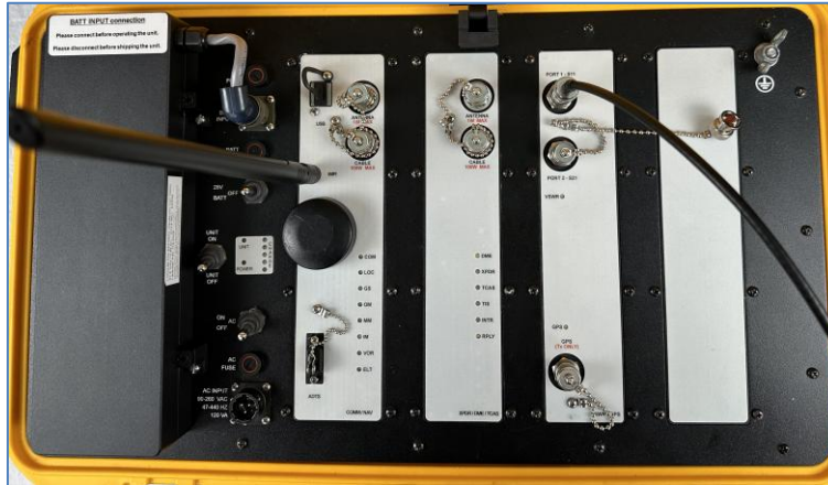
VSWR Setup with connection to Port 1
