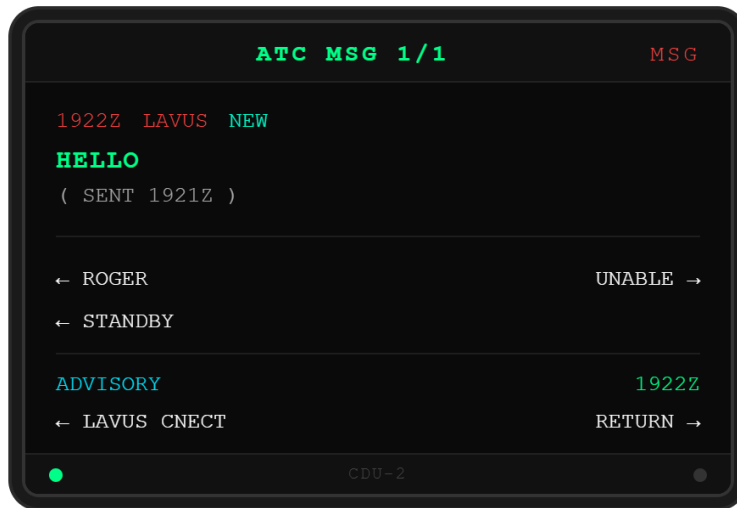
HELLO Message received by the aircraft using the Datalink VDLM2 interface
