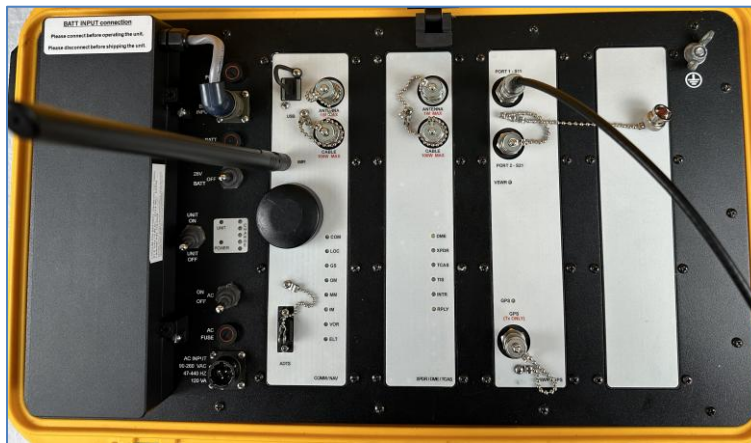
VSWR Setup with connection to Port 1
