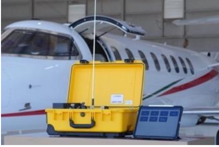
1. NAV/COM Telescopic Antenna in operation on an ARTS 7000 Test Set
