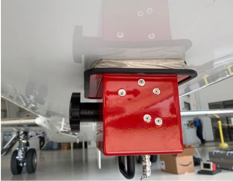
Coupler in position on the bottom antenna. In this case the coupler is being used as a shield – note the termination is connected on the coupler connector.
