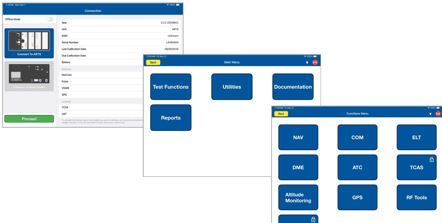
Each test function has a dedicated page giving the operator full access to test parameters, configuration, and results. All test functions can be setup and completed by a single technician. The familiarity of tablets and the simplicity of the ARTS software minimizes training time. If you can use a tablet, you can operate the ARTS.
