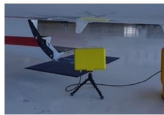
Good line of sight between Aircraft Antenna under test and ARTS 7000 test antenna.
