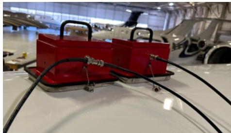
ARTS 7000 GPS couplers covering dual aircraft antennae.
