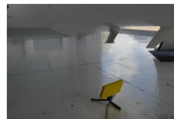
Good line of sight between Aircraft Antenna under test and ARTS 7000 test antenna.
