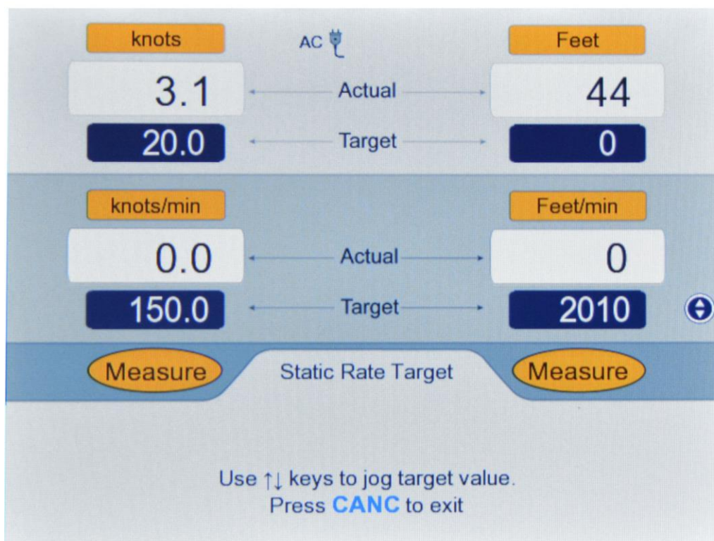
Figure 3.14 : Jog the Static Rate Target value
