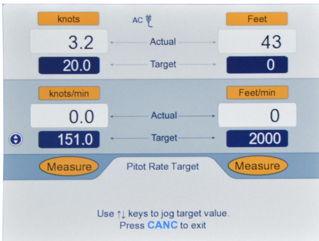
Figure 3.12 : Jog the Pitot Rate Target value
