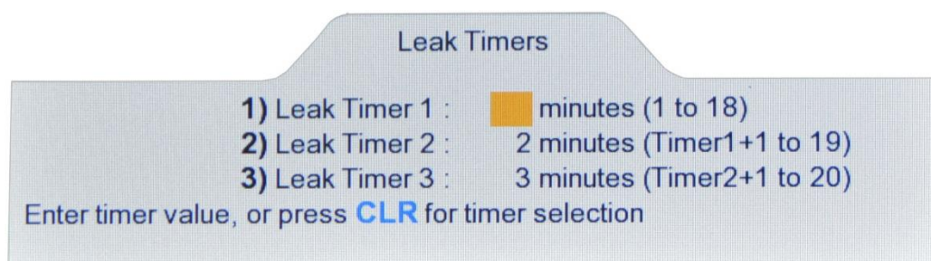
Figure 3.49 : Adjust Leak Timer
