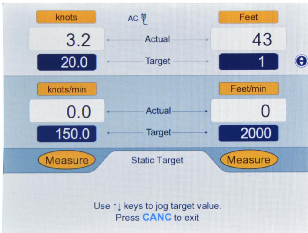
Figure 3.10 : Jog the Static Target value
